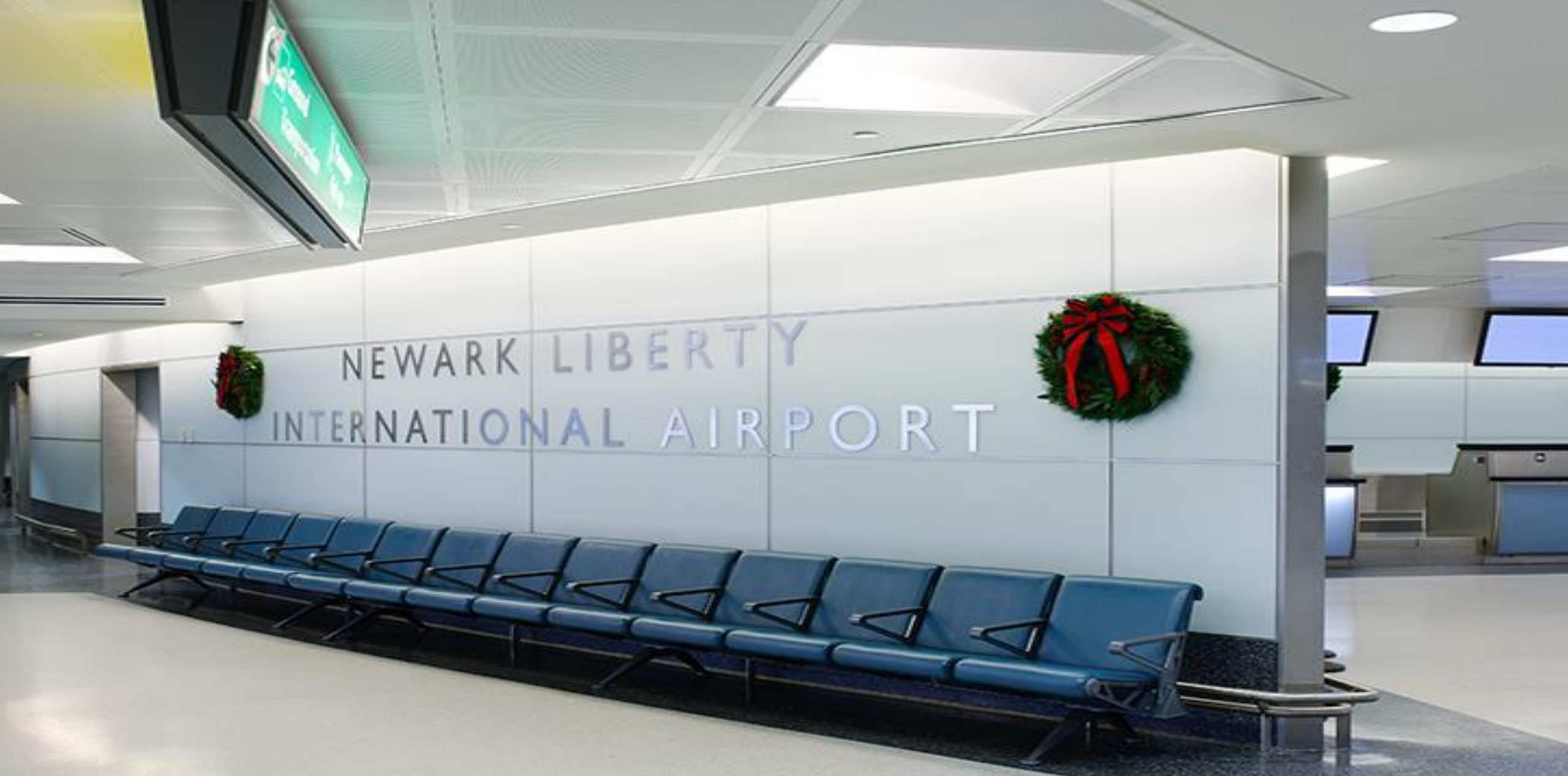
Newark Airport – Newark, NJ 6mm clear acid-etched glass, tempered & laminated
